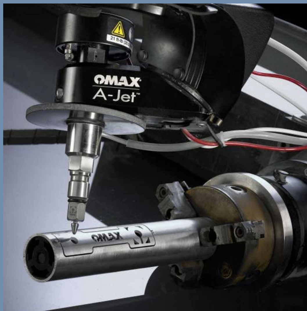
OMAX A-Jet with Rotary Axis enables 6 axis cutting.
