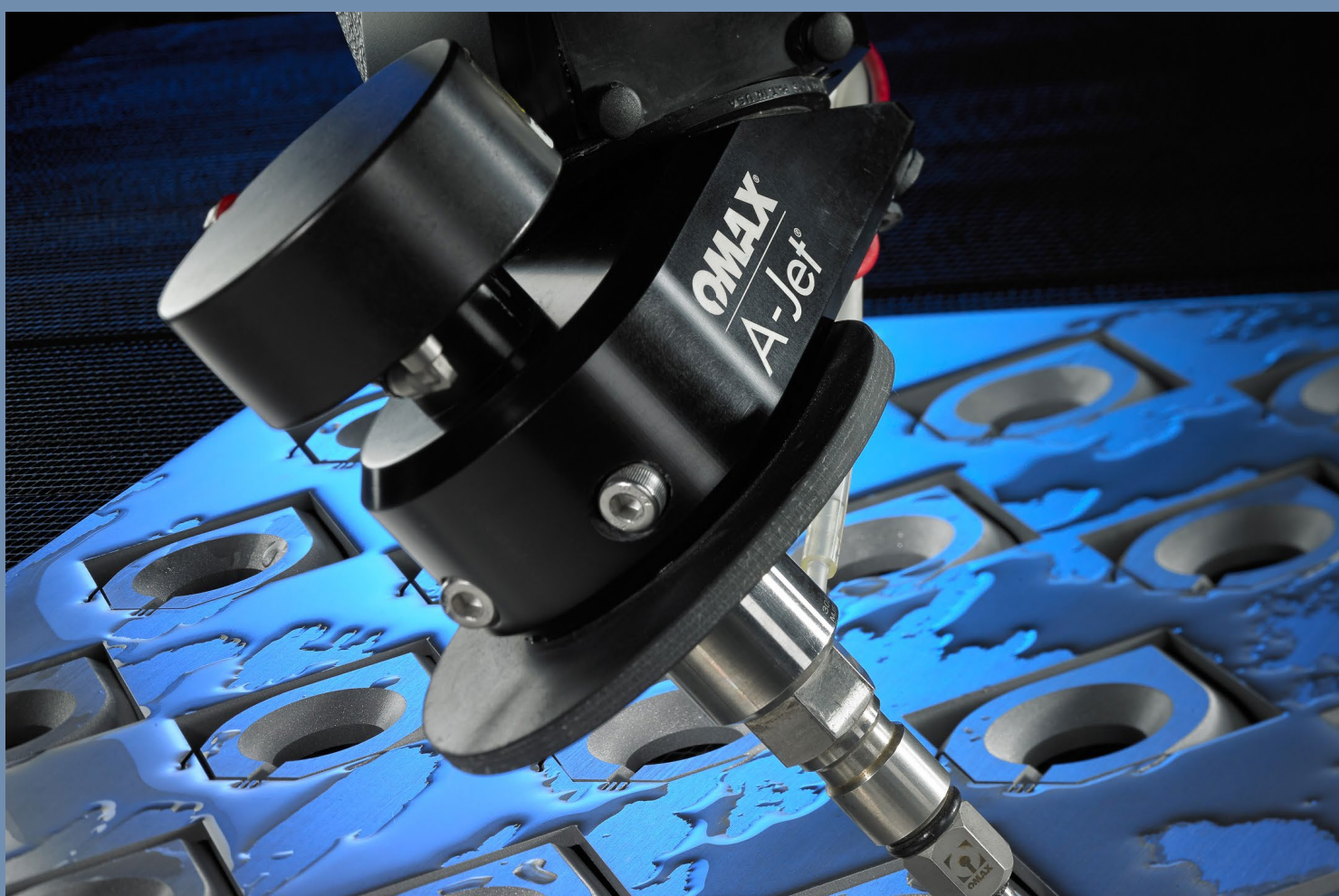
OMAX A-jet provides 5 axis cutting capabilities.
